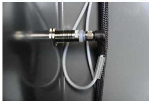
Figure 2. Sonic Sensor or Sense Car in the base of the Auto Sentry flex HD
