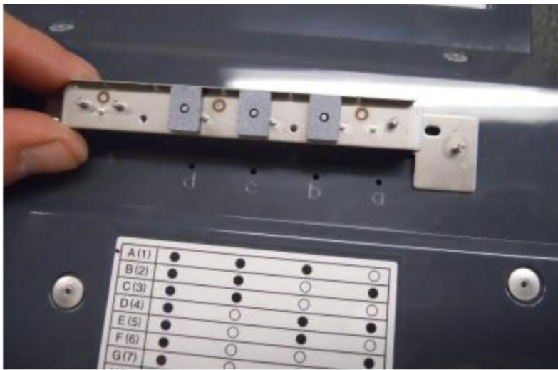
MAGNETS IN POSITION A(1)
